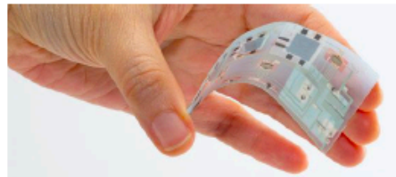
Smart label w/ printed memory technology licensed to Xerox
